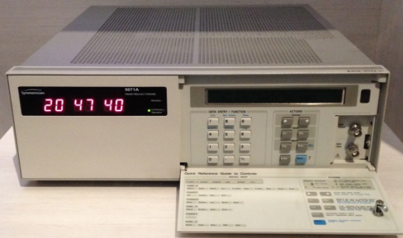
Cesium Frequency Standard (Atomic Clock) 2012
